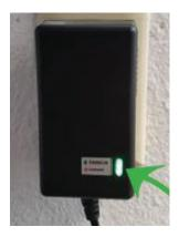
Place the battery in the charging cradle. If the battery is up to charged voltage, the LED on the charger will stay green. If the charger determines that the battery needs to be charged, the LED on the charger will change to red.
