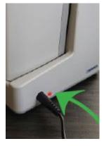
**NOTE:** If the battery light is green but your lift is inoperable, it is possible that the battery is no longer able to hold a charge. Please check the battery voltage with a voltage meter. A fully charged battery is 24+ volts. If the voltage is low, contact us to discuss repair or replacement options.
