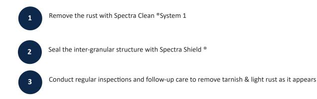
Long-term protection for surfaces of new and old stainless steel can be attained by applying Spectra Shield <sup>®</sup>to the surface after removing the rust and drying the surface. This forms a protective layer in the pits and inter-granular boundaries that prevents air and water from creating corrosion below the surface. Without oxygen and salts from pool water making contact with the stainless steel, the rust will not grow.
