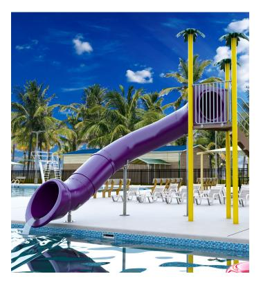
Single flume triangle deck poolside slide features a single 90 ° enclosed slide flume, a triangle deck, and center steps with rails. The slide flume is fabricated from rotationally molded UV stabilized color impregnated LDPE. Custom colors are available.
